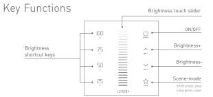
★ When blue indicator light of <sup>()</sup> key is on, long press <sup>()</sup> to turn on/off buzzer. When white indicator light of <sup>()</sup> key is on, long press <sup>()</sup> to match code.
